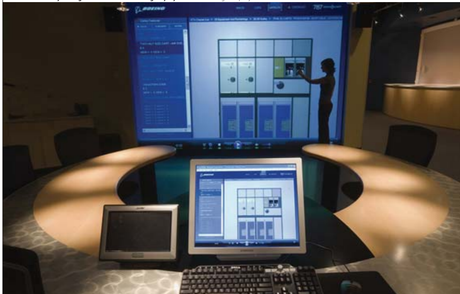
A full-height, backlit screen in the galley showroom for the 787 Dreamliner allows customers to view different galley configurations ‘virtually’. In this way, they can test and study the ergonomics of their chosen galley layouts © The Boeing Company
